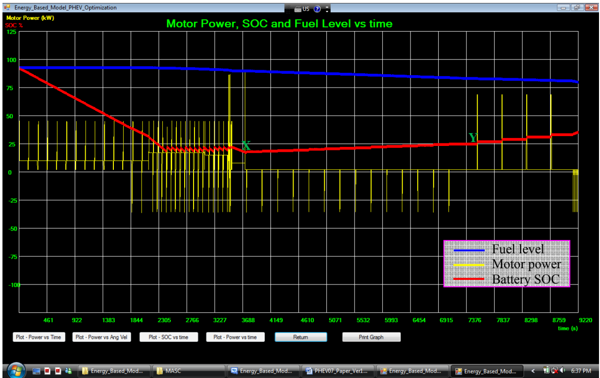
Fig. 6: Motor power, SOC and fuel level versus time for entire journey.
